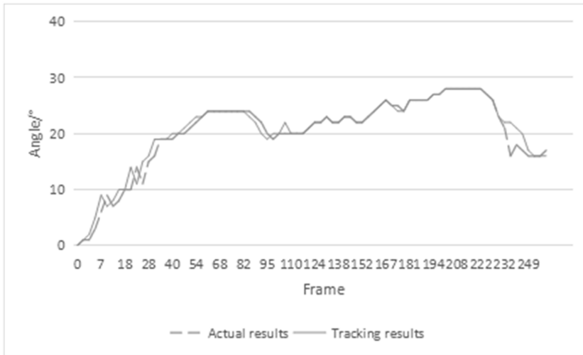
Fig. 5. Comparison of tracking results and real values of synthetic sequences between human hand and sphere: angle of thumb TM joint flexion
